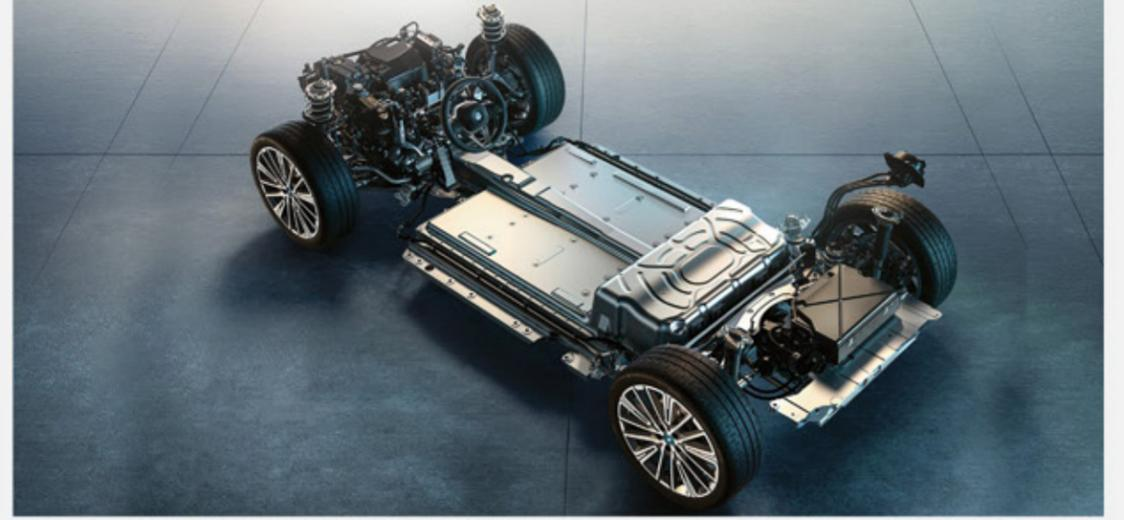
**M Adaptive Suspension:** Dynamic Damper Control, frequency-selective damping elements: mechanical, self-regulating system with regulation depending on road condition and driving style, also includes M Sport steering which allows for more direct steering feedback with lower steering effort. (only for iX1)
