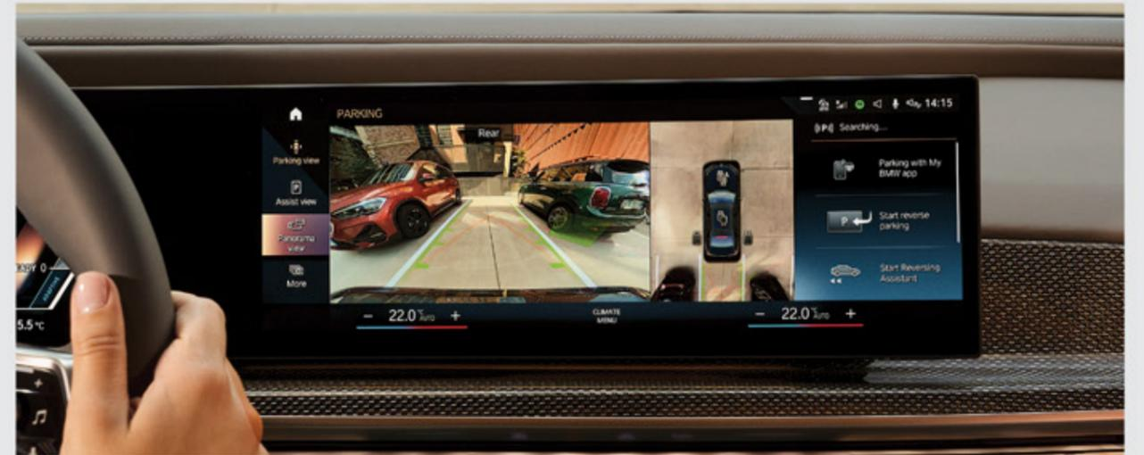
**Parking Assistant Plus:** Visual parking aid featuring surround view cameras, Top View, Panoramic View and 3D View makes parallel and perpendicular parking to the road easier. The system completely takes over the steering, the accelerator, and the transmission.
