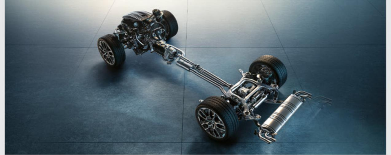
**Adaptive M Suspension Professional:** Combines Active Roll Stabilization with Integral Active Steering, so the movements of the vehicle's superstructure when driving in turns and on straights is reduced to a minimum (Only for the M60i Variant).
