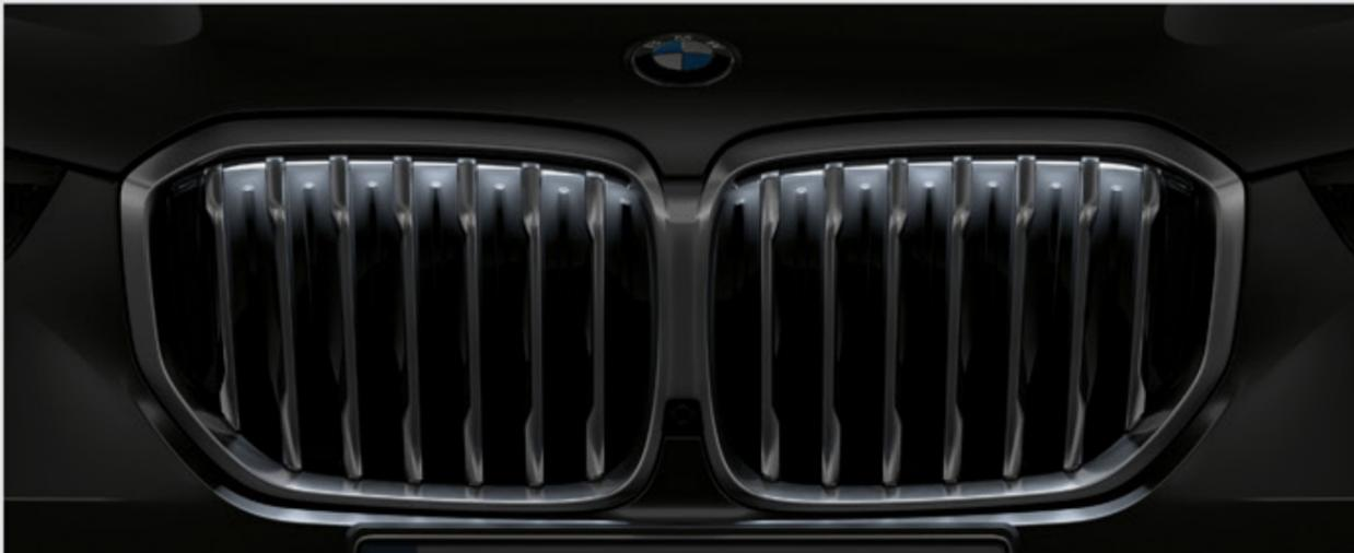
**BMW "Iconic Glow" active kidney grille:** Highlighting of BMW radiator grille by innovative LED fibre optical technology "Active" indicates the opening and closing of the air vents to actively regulate the airstream. They close for increased aerodynamics and open if the cooling demand for the engine increases (Only for the xDrive40i Variant).
