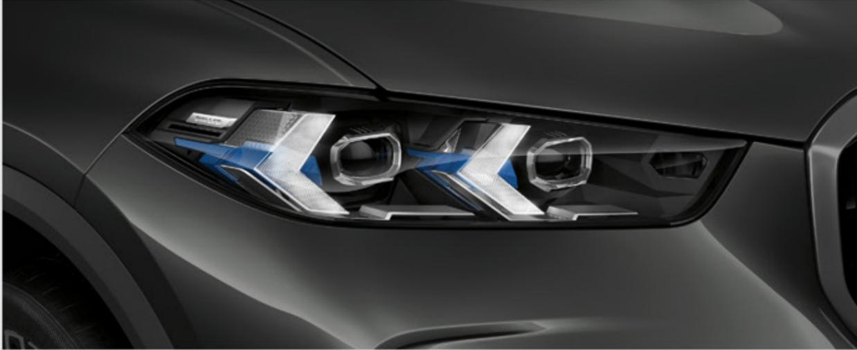
**Adaptive LED Headlights** with cornering lights offer a bright and efficient bi-LED light for low beam and high beam featuring BMW Selective Beam and High Beam Assistance.
