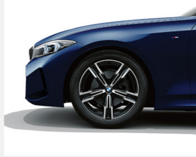
18" M light alloy wheels Double-spoke style 848 M Bicolour with run-flat tyres.
