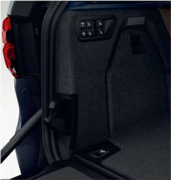
Luggage control unit: electric folding of the seats in the 2 nd and 3 rd seat row, with integrated buttons to get maximum luggage capacity or maximum seating.
