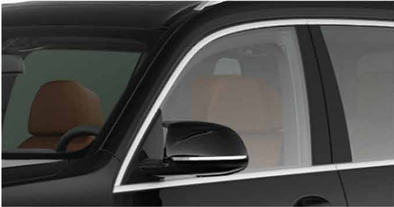
Acoustic Glazing: sound-insulating glass which increases driving comfort.
