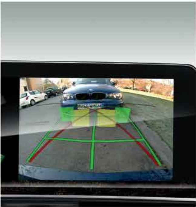
Parking Assistant: includes rear view camera with front and rear sensors, allows automatic parallel or perpendicular parking.
