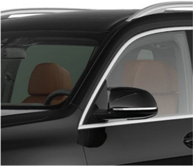
Acoustic Glazing: sound-insulating glass which increases driving comfort.
