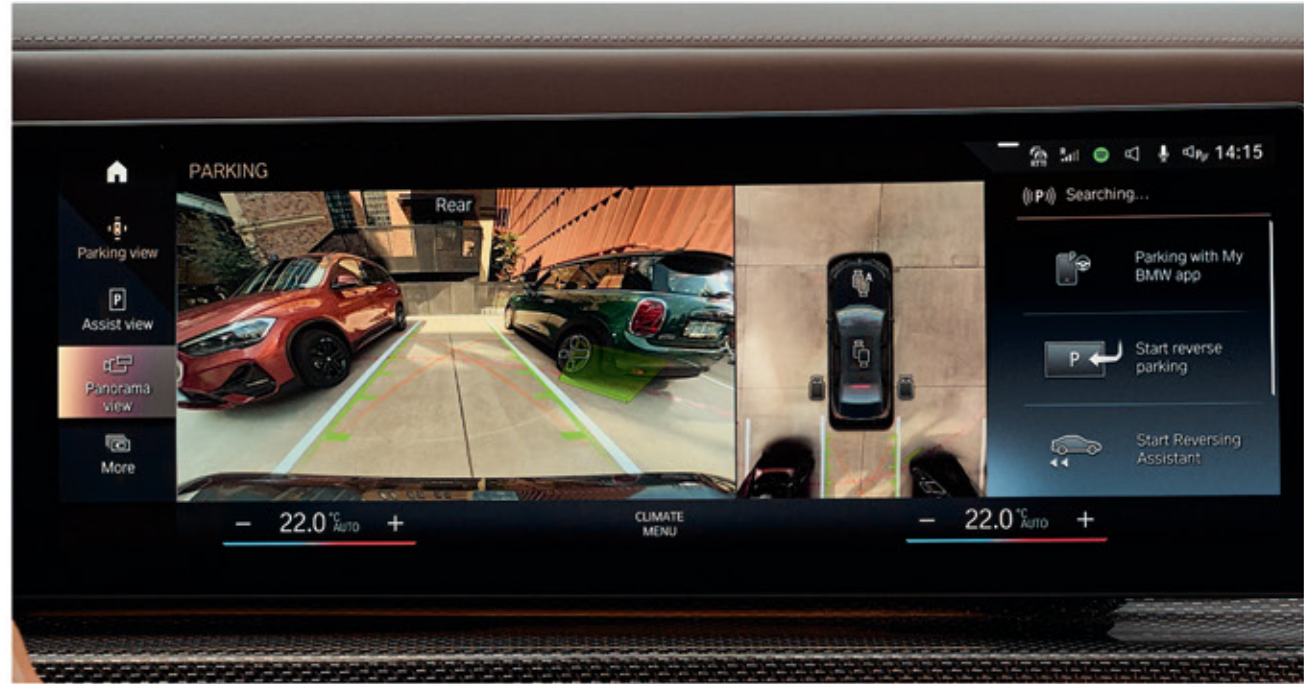
Parking Assistant Plus: Visual parking aid featuring Rear-view Camera, Top View, Panoramic View and 3D View makes parallel and perpendicular parking to the road easier. The system completely takes over the steering, the accelerator, and the transmission.
