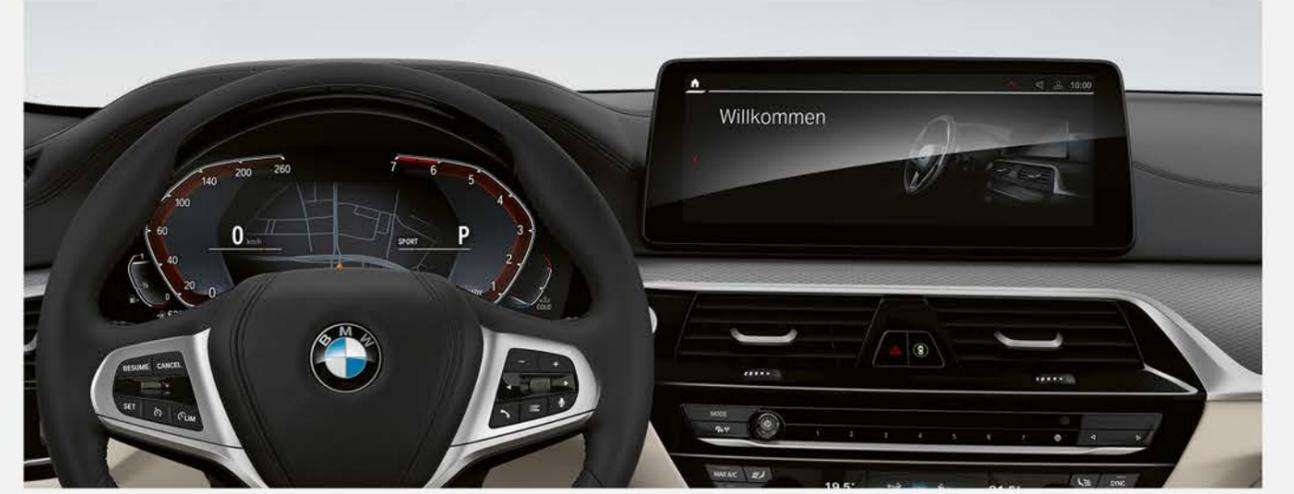
**BMW Live Cockpit Professional:** with navigation function includes a high-quality display network consisting of a high-resolution 12.3" Info Display that can be operated by touch and a fully digital 12.3" instrument cluster.
