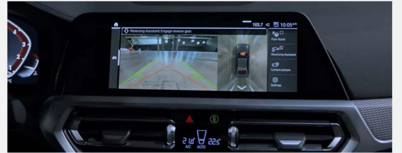
**Parking Assistant Plus:** visual parking aid, featuring Rear-view Camera, Top View, Panorama View and 3D View, makes parallel and perpendicular parking to the road easier. The system completely takes over the steering, the accelerator and the transmission.
