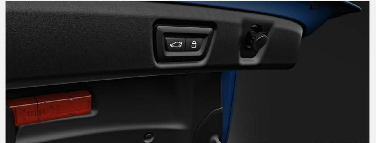
**Automatic operation of tailgate:** Remote opening with key, closing by tailgate button or remote control.
