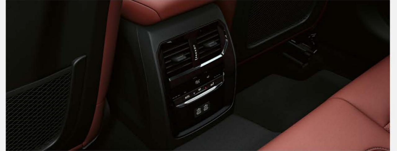
**4-Zone Automatic Air Conditioning:** includes separate control element with display in the rear for individual temperature setting as well as air vents in the B-pillar.
