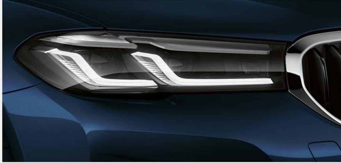
**Adaptive LED Headlights** The LED headlights with cornering lights offer a bright and efficient bi-LED light for low-beam and high-beam headlight functions.
