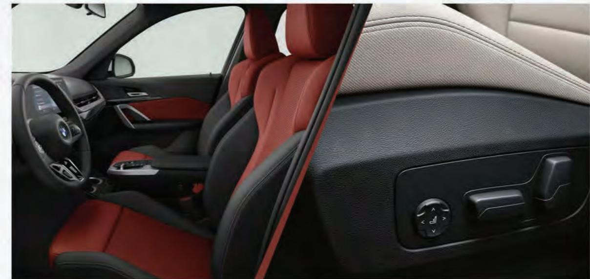
**Sport seats** for driver and front passenger with electronic adjustment.
