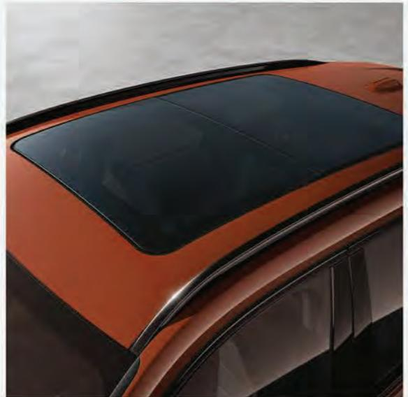
**Panoramic glass roof:** Electronic sliding and tilting functions.
