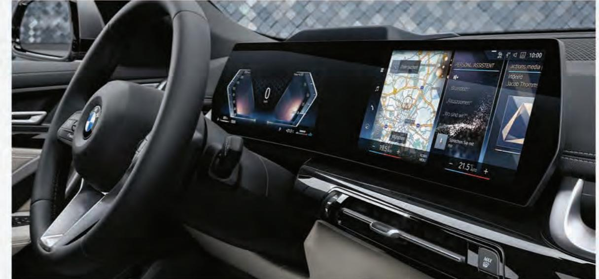
**BMW Live Cockpit Plus** with navigation functionality includes a high-quality display curved screen consisting of a high-resolution Display Cluster consisting of a fully digital 10.7" Instrument Display and a high-resolution 10.25" Control Display.
