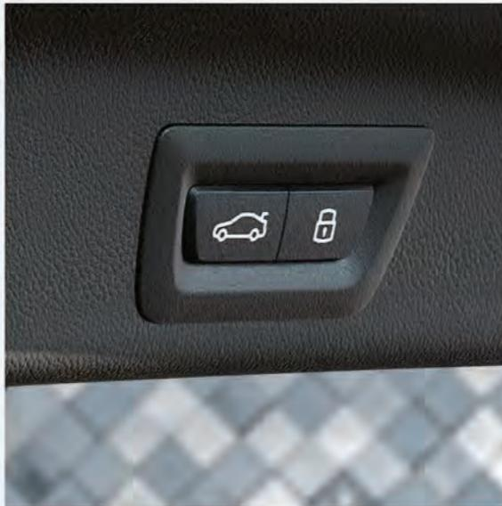
**Automatic operation of tailgate:** Remote opening with key, closing by tailgate button or remote control.
