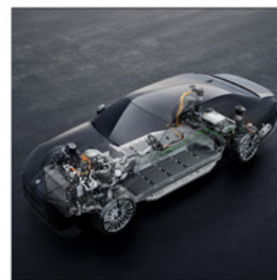
The Adaptive Chassis Control Professional combines active roll comfort, active roll stabilization, adaptive two-axe air suspension, and integral active steering to deliver a composed and balanced driving experience. The system continuously works to enhance ride comfort, stability and steering precision across different driving conditions.
